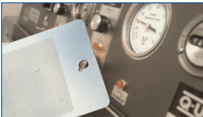
Xylan 1514 after 225 hours QUV (ASTM G-53) exposure. The coating shows only a 5% shift in gloss.
