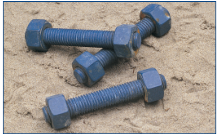
Xylan 1014 after 1,080 hours of exposure in the salt fog cabinet. Rust is minimal, the coating is still functional and the fasteners are fully serviceable.
