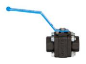
**225SGS** Carbon steel 800LB ball valve, suitable for 136 bar at 38°C/10 bar at 200°C.
