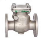
Stainless steel 200lb/in<sup>2</sup> check valve, suitable for 13,8 bar up to 177°C.
