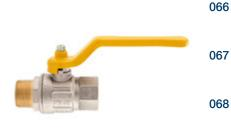
**LONDON 'GAS' nickel plated brass ball valve,** suitable for up to 5 bar at 60°C. Full bore, chrome plated brass ball, PTFE seats, standard lever, screwed BSP (FxF). 8mm to 50mm
