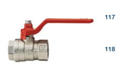
**VIENNA nickel plated brass ball valve,** suitable for up to 50 bar at 20°C/12 bar at 150°C. Standard bore, chrome plated brass ball, PTFE seats, standard lever, screwed BSP (MxF).
