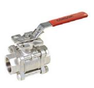
300S Stainless steel ball valve, suitable for 69 bar at 38°C/5 bar at 200°C.
